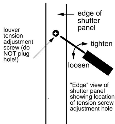
11. All shutter panels come with "tension" screws deeply counter-sunk in each vertical edge. By simply turning the screw a little clockwise or counter-clockwise with your Phillips head screwdriver, you can gently tighten or loosen the louver/pushrod tension in each individual panel to suit your preferences. When adjusting the tension, always spread the amount of adjustment evenly between all screws in BOTH edges of the individual panel (see figure above, right).
