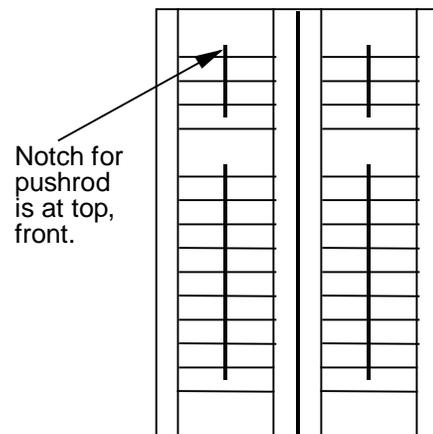
3. Install shutter panels with the “notch” for the pushrod at the TOP. When installed, the pushrod faces the room. (See Figure “A”)
